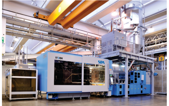
96 Cavity preform moulding machine with hopper, drier and de humidifier.
